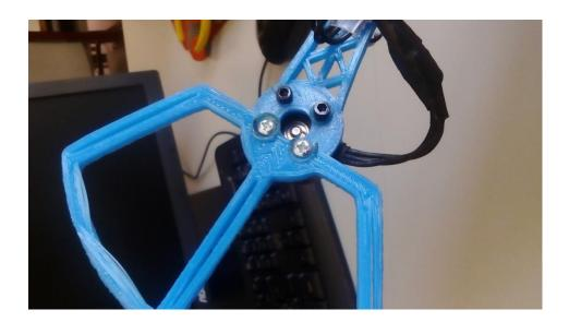
The basic structure of the drone can be bought online or downloaded in STL files to modify, redesign and print to a 3D printer.
