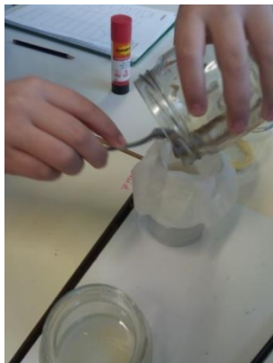
05 Heterogeneous mixtures can be separated by filtration
